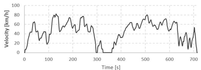
Figure 10: Reference velocity profile of the leading vehicle used for real world experiment.
