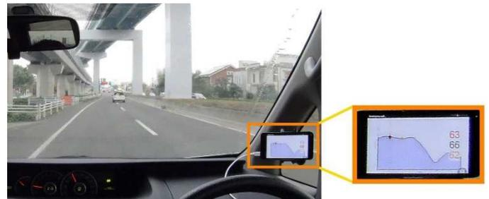
Figure 9: View from the driver of the leading vehicle. The velocity profile display system is squared and zoomed on the right. Current velocity, future velocity and velocity plot were displayed.
