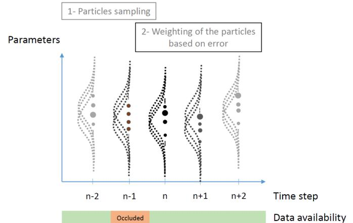
Figure 1: Parameter identification process steps 1 and 2
